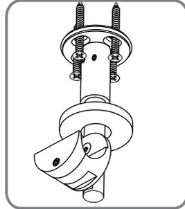
Slide trim plate down. Secure to ceiling with screws properly anchored to the substrate.
