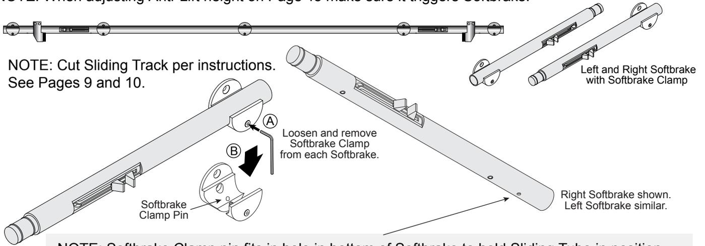
NOTE: Softbrake Clamp pin fits in hole in bottom of Softbrake to hold Sliding Tube in position. Install Softbrake Clamps after Wall Clamps are installed to ensure proper location. Follow Steps 1 through 4 on Pages 11 and 12 to install Wall Clamps and Sliding Tube.
