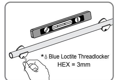
When Tube is level, tighten the Glass Clamps.
