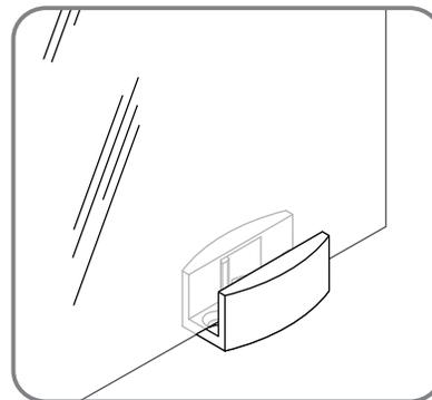
Hang door again making sure it is engaged with the floor guide.
