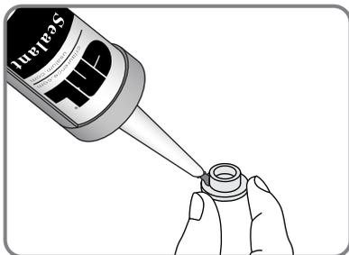
Use a dab of RTV408C silicone to hold cap in place.
