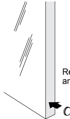
Remove from backing and place on door edge.
