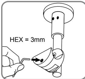
Loosen clamp to install sliding tube.
